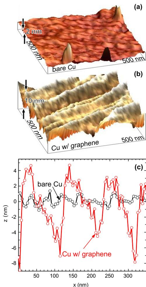
Figure 1. Atomic force microscopy micrographs of copper (a) with and (b) without the growth of graphene. Note that sample (a) underwent the same process as (b) just without CH<sub>4</sub> flow. (c) shows line scans of the corresponding surfaces depicted in (a) and (b).
